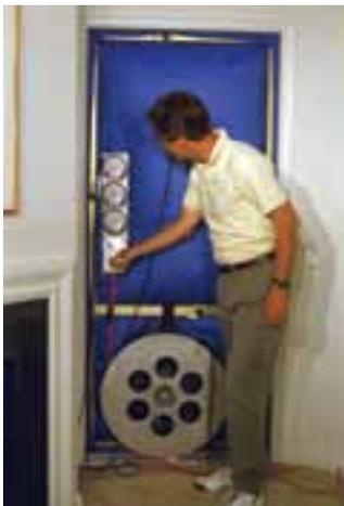
A blower-door test finds leaks that can be sealed, creating an airtight building with minimal heat and air-conditioning loss.
